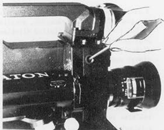
positioning the retractable beam splitter.
