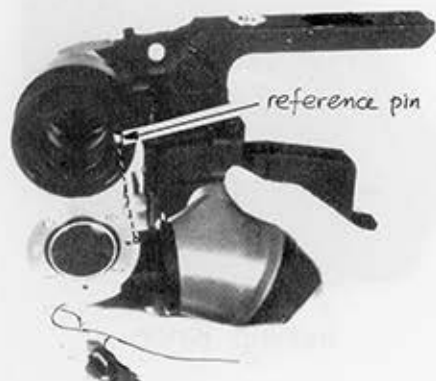
placing short and long eyepieces onto viewfinder
