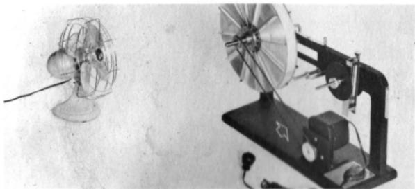
The Drying motor should be fastened to the base of the loading stand as shown in the above figure. Use the two open slots provided in the base, and place the two mounting strips underneath the base, inserting the four mounting screws into the tapped holes in the strips. Adjust the position of the motor to accommodate 16mm, 35mm, 70mm, or whatever size reel is being used, and then tighten down the four mounting screws to fasten the motor firmly in place.
