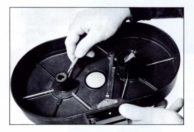
Remove the set-screw from the feed spool-holder, as shown at left. Then remove the set-screw from the collapsible take-up core. Both cores can now be removed from their shafts.
