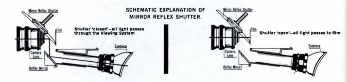
Heart of the Arriflex reflex system, as diagrammed above, is the segmented mirror-shutter which rotates at a 45° angle between the lens and the filmplane. When the shutter is closed, the image is reflected off the mirror segments into the viewfinder. When the shutter is open, all of the light passes between the segments directly into the film. Thus the system is a time-sharing arrangement and no beam splitter is used.
