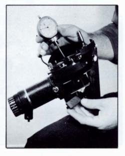
Since all lenses used on Arriflex cameras are adjusted for exactly 52mm, the question arises as to why the distance from the turret surface to the film aperture should be 52mm -0.03. The reason for the minus tolerance is that most film is not perfectly flat, but tends to curve slightly away from the lens. Degree of curvature may vary depending upon type and age of the film. By compen – sating for this curvature, perfect sharpness will be obtained.
