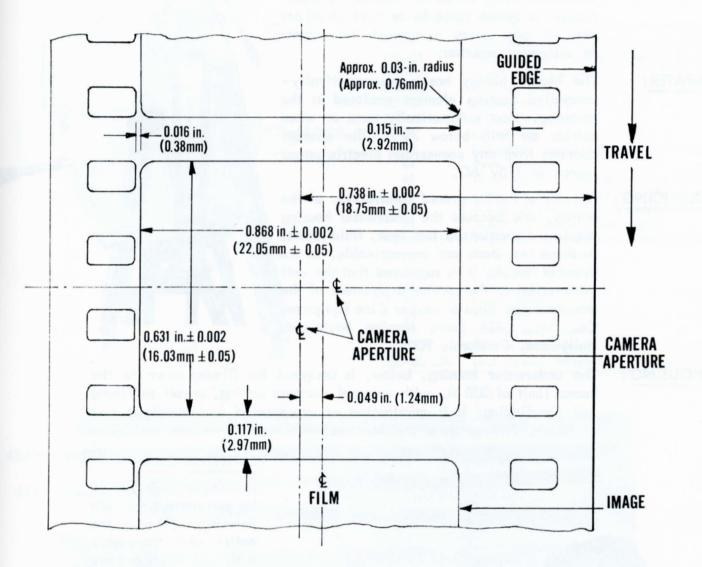
Dimensions given (in both inches and millimeters) apply to unshrunk raw stock. Aperture dimensions shown, in combination with an  $0.600" \times 0.825"$ (15.25 x 20.95mm) projector aperture, will produce a screened picture with height-to-width ratio of 3 to 4 at a projection angle of 14 degrees.
