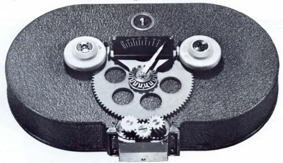
REMOVAL OF SPROCKET HOUSING: Remove four screws 10-65. Unhook spring 10-40. The sprocket assembly as a unit can now be pulled out from the magazine casting.
