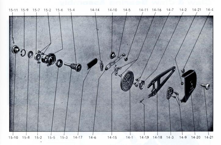
Cardioid cam claw system with claw bearing
