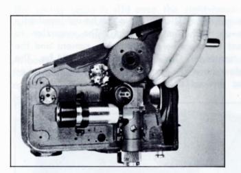
The intermediate gear can now be taken off, as shown in lower photo at left.
