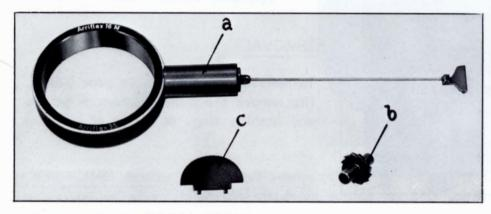
Special tools used include (a) spring scale, (b) auxiliary ratchet wheel, and (c) wrench.
