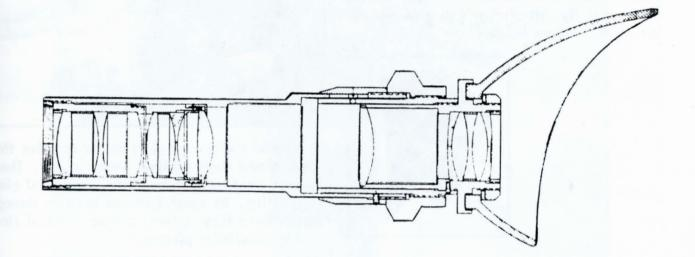
The viewfinder as a unit should not be disassembled. If any optical elements are damaged, it might be necessary to replace the entire finder assembly. At any rate, any repairing should be done only by an experienced optical technician.
