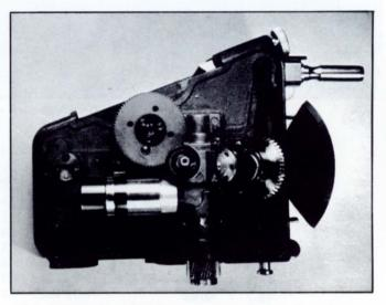
The left edge of the center rib of the shutter should line up with the right edge of the claw. When the claw and mirror are lined up as described, then the timing will be correct.
