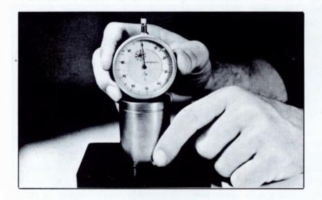
Hold the parallel steel block firmly against the film aperture plate, and place the dial indicator into the open lens socket, as shown at right. Make sure that the matching surfaces of the dial and lens socket are clean.
