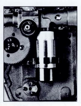
IMPORTANT: The connecting gears between the tachometer and the drive shaft must have proper play.
