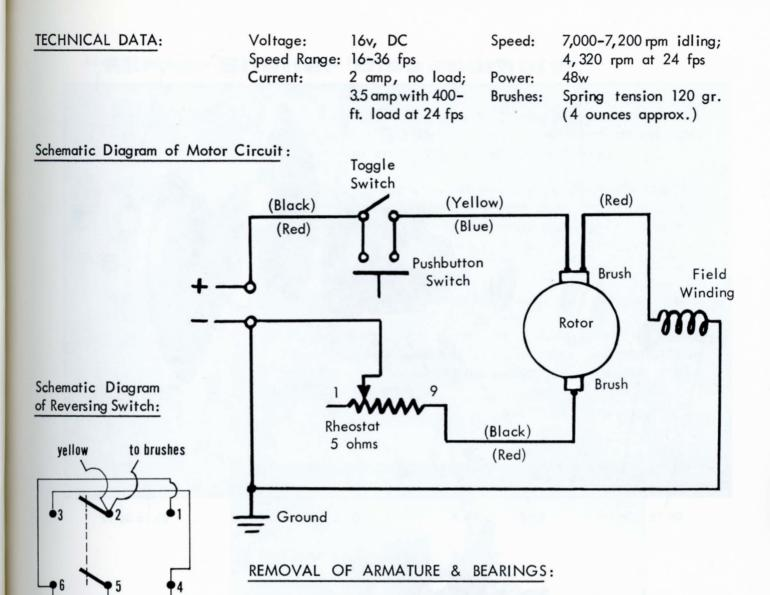
On cameras with reversing-type motors, rheostat housing can't be removed until five wires leading to reversing switch have been disconnected. (It is not necessary to disconnect the jumper wires between poles 1-6 and 3-4.) When reassembling, use the diagram above.
