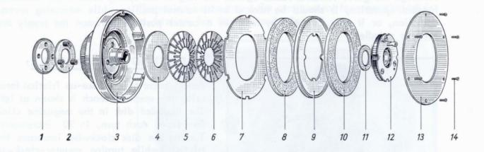
(1) Threaded Disk; (2) Ratchet Disk; (3) Housing; (4) Pressure Plare; (5)(6) Disk-shaped Tension Springs, convex surfaces facing; (7) Pressure Plate; (8) Felt Ring; (9) Friction Plate; (10) Felt Ring; (11) Separator Disk; (12) Ratchet Carrier; (13) Cover Disk; (14) Countersunk Screws.
