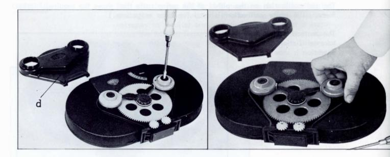
The magazine cover (d) is removed by loosening its mounting screws. Then the cylinder head screw which holds the friction unit at the center of the spindle is removed, as shown above left. Finally the unit is lifted up in one piece, as shown above right. Individual parts of the friction unit assembly are shown below:
