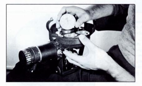
To obtain perfect focus and sharp pictures, the flange focal distance must be kept in strict tolerance.
