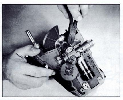
above, is the segmented mirror-shutter which ratates at a 45° cogle between the lens and the filmplane. When the shutter is closed the inege is reflected off the mirror segments into the viewinder. When the shutter is open, all of the light passes between the segments directly into the film. From the system is a time-shoring arrangement and no beam splitter is used.
