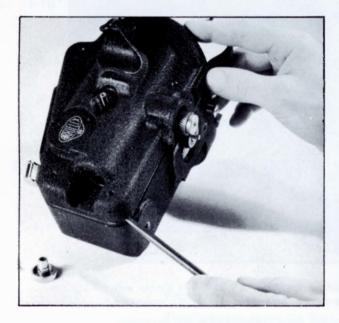
If the cover has a tight fit, use screwdriver or knife blade as shown above.
