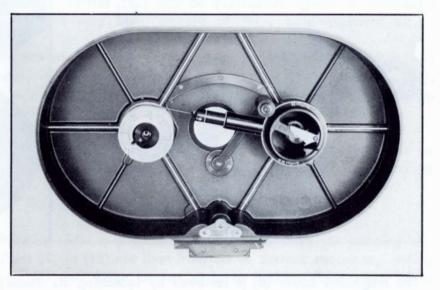
The spring scale is slid over the right-hand core and the flat hook at the end of the nylon cord is threaded into the film-holding slot of the left-hand core. The motor is run in reverse at 24 fps.
