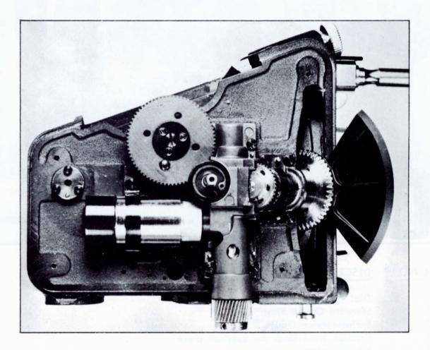
When the camera gear assembly is exposed, as shown above, it can be checked, cleaned and lubricated.
