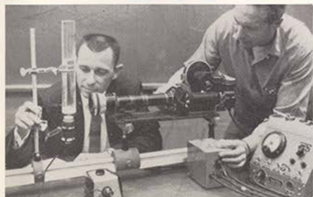
© FRED ALLEN (LEFT), CHIEF OF THE CRYSTAL GROWTH SECTION, BASIC RESEARCH GROUP AND GENEVY L. FILLMAN, MOTION PICTURE SPECIALIST, SET UP ARRIFLEX IN WITH BENCH MOUNT KILN AND LONG EXTENSION TUBES FOR TIME-LAPSE MONITORING OF CRYSTAL GROWTH.
