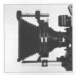
The light-weight matte box is fixed on to the front of the lens. An adapter ring corresponding to the lens diameter ensures that it is firmly seated. For zoom lenses (with the exception of the Zeiss-Vario-Sonnar f 1,8 10—100) a round rubber hood should be used as a sun shade; for fixed focal length lenses, and the before-mentioned Zeiss-Vario-Sonnar, a rectangular rubber tube should be used. As the light-weight matte
