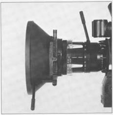
box is used mainly for news gathering, a rotatable filter stage is unnecessary. A holder takes two 3" x 3" filter frames. When using the Vario-Sonnar f 2,8 10—100, to ensure smooth focussing, the focus lever is displaced forwards by means of a detachable extension. (See also Technical Information ARRIFLEX Light-Weight Matte Box).
