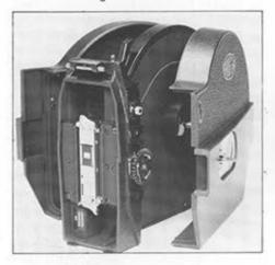
A quartz controlled 12 V DC motor is installed to drive the camera. Frame rates of 24 and 25 fps can be selected. Pilot frequencies of between 50 and 60 Hz, proportional to the camera motor speed, can also be selected. Synchronous double system recording is possible with this camera using the following methods:
