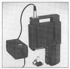
The Energy Set is comprised of the NC 12/4E camera battery with a capacity of 4 Ah, with automatic cut-out and the fully insulated NCL 12/4E battery charger for accelerated charging with automatic 110/220 V mains voltage selection. The charging unit can be switched over from 50/60 Hz. The impact-resistant hard rubber housing of both units provides excellent protection under the roughest conditions. The battery has a carrying handle or can be attached to the cameraman's belt or shoulder strap.
