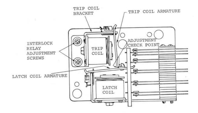
FUNCTIONALLY, THIS TYPE OF RELAY IS THE SAME AS OTHER RELAYS, DIFFERENT ONLY IN THAT IT IS 'LOCKED IN' MECHANICALLY ALTHOUGH THE COIL IS DE-ENERGIZED.
