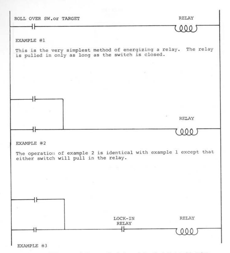
The only difference with example 3 from 2 is that the hold relay switch must be closed to complete the circuit.
