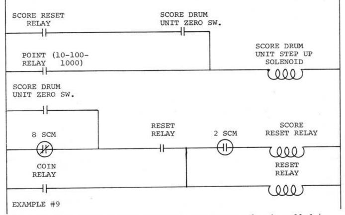
When the coin relay switch is closed, the reset relay is pulled in starting the score motor. The reset relay will stay locked in until all the score drum units advance to zero, and when #8 score motor cam switch is actuated. As long as the reset relay is energized, the score reset relay will pulse thru #2 score motor cam. During the game reset time the score drum units will advance until the score drum units zero switch opens.
