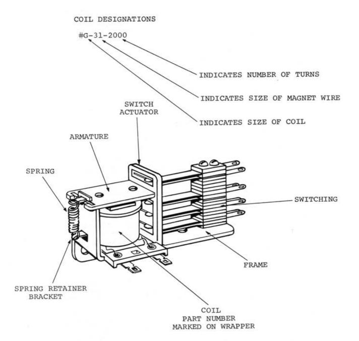
TIGHTEN DOWN THE SCREWS THAT HOLD THE SWITCH ASSEMBLY. THIS IS SUGGESTED BECAUSE THE PLASTIC SPACERS IN THE SWITCH STACKS WILL OCCASIONALLY SHRINK BY DRYING OUT, CAUSING A POOR ADJUSTMENT.
