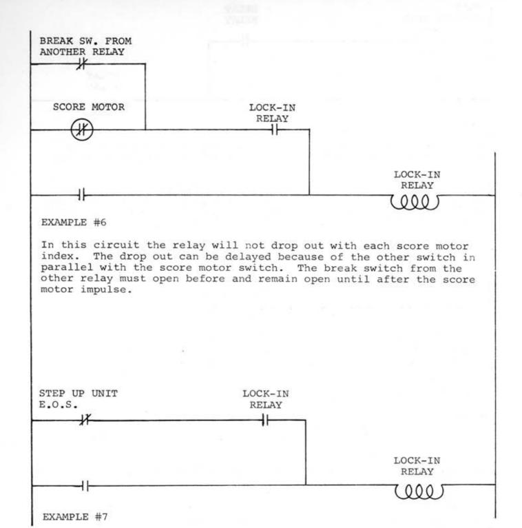
The relay is locked in through a step up unit end of stroke switch. The step up unit must advance for the relay to drop out. A typical example of this circuit is in the point relay (10,100,1000) lock in circuits.
